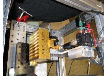
Figure Four: (left) A 1x8 mixer module fully assembled (top) and top removed (bottom) (right) The Supercam 64 pixel Lo divider block
